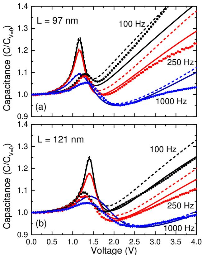
Figure 2. Capacitance  $C$ , normalized to its value at  $V = 0$ , as a function of  $V$  at different frequencies for (a) the  $L = 97$  nm and (b) the  $L = 121$  nm device. Dots: measurements.<sup>12</sup> Full (dashed) lines: simulation results for  $\sigma = 0.08$  eV and a SC (FCC) lattice.
